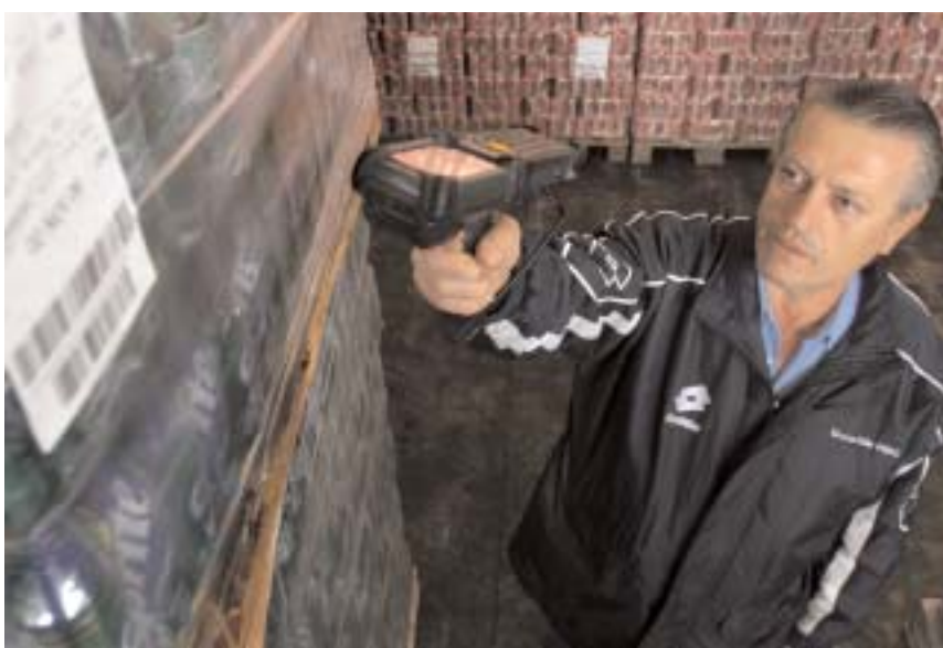
A traceability system for product pallets has been developed and installed in all Coca-Cola HBC production plants, warehouses and depots within the European Union. The system uses a label with unique production information and wireless scanning guns.
